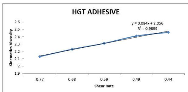
Fig. 3 Rheological analysis of gelatine-based adhesive formulated from cow hide.
