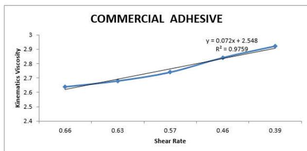
Fig. 4 Rheological analysis of commercial-based adhesive.
