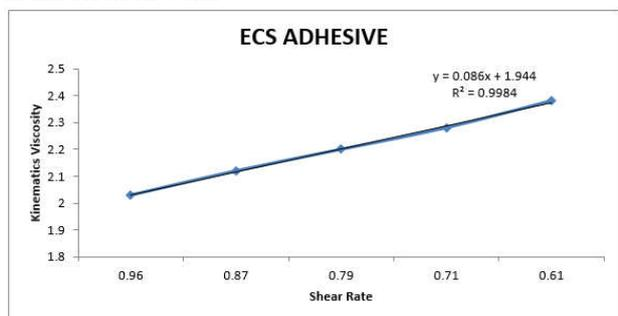
Fig. 2 Rheological analysis of starch-based adhesive formulated from Eleusine coracana.
